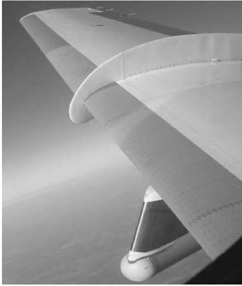
Fig. 24 Starboard airfoil with parylene-coated multisensor hot-film array in flight.
