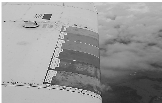
Fig. 13 Multisensor hot-film arrays on a Piper 28 airplane (altitude, 3000 ms; airspeed, 130 kn; air temperature, -10^{\circ}\text{C} ). From top to bottom: ZnO-coated hot film, polyimide-coated hot film, parylene-coated hot film, \text{SiO}_x -coated hot film, and two pure hot films.
